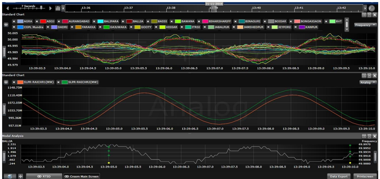
Fig-1: Frequency at different 400kV buses and 765kV Raichur-Sholapur line flow
